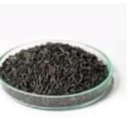
molecular sieves belong to the group of microporous materials aracterized by the relatively high adsorption capacity and selectivity towards a wide spectru gases. They posses amorphous structure with well developed surface area and the pore simparable to the effective diameter of small molecules
