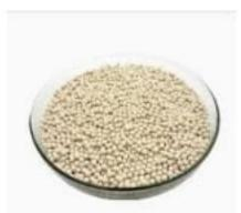
Molecular sieves are used for drying gases and liquids and for separating molecules on the basis of their sizes and shapes. When two molecules are equally small and can enter the pores, separation is based on the polarity (charge separation) of the molecule, the more polar molecule being preferential adsorbed.
